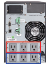
This Eaton 9130 UPS is equipped with two load segments, each with three 5-15R
